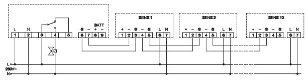
Notes: (1) The remote sensors used are: **SGAMET, SGAGPL, SGIME1, SGIGP1, SGIME1M, SGIGP1M**. (2) The back-up battery to be used is ACCSGB12.
